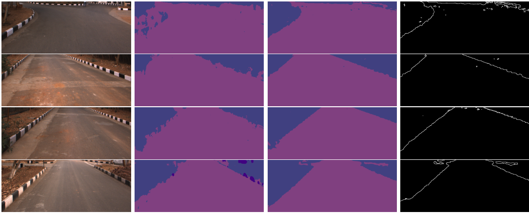
Figure 6: We show results for various tough outdoor scenarios. The first column is the left image from stereo camera , second column shows the SegNet results, third column is the final CRF output, forth column shows the curb boundaries by applying canny edge detection on the CRF output
